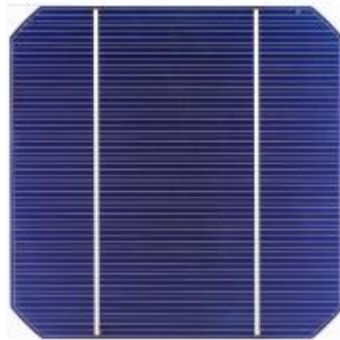
Figure (I-6): Cellule en silicium monocristallin [16].
