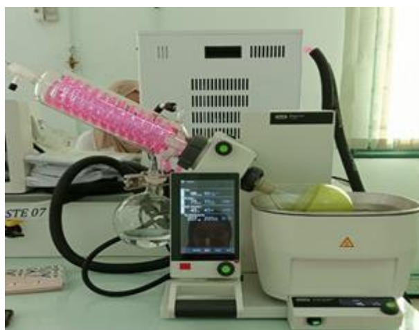
Figure 19: Ethanol evaporation process using Rotary Evaporator(This is a personal photo).
