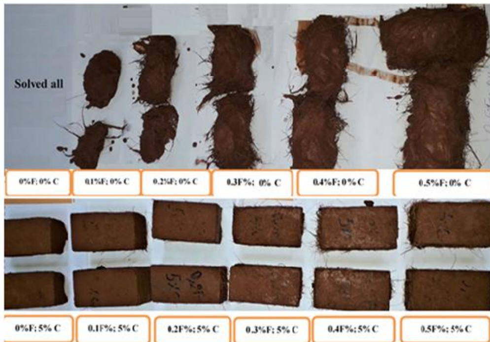
Figure IV 5: Appearance of blocks after water immersion
