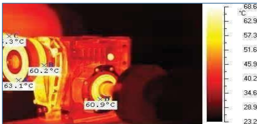
Figure II.3. Thermo gramme : usure de palier
