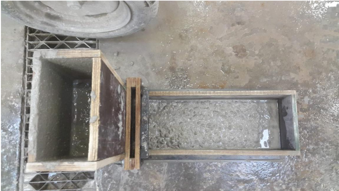
Figure V-15. Blockage of SCCFA3 based on fly ash.
