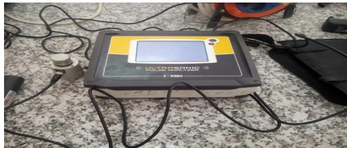
Figure III-4. Ultrasonic pulse velocity test device.
