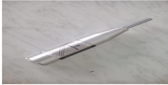
Figure III-3. Rebound hammer test (Sclerometer).
