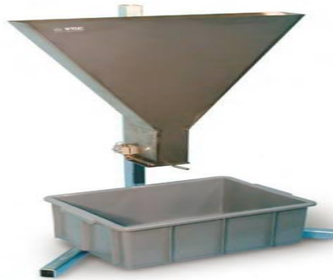
Figure II-2. V-funnel test (NF EN 12350-9, 2010).
