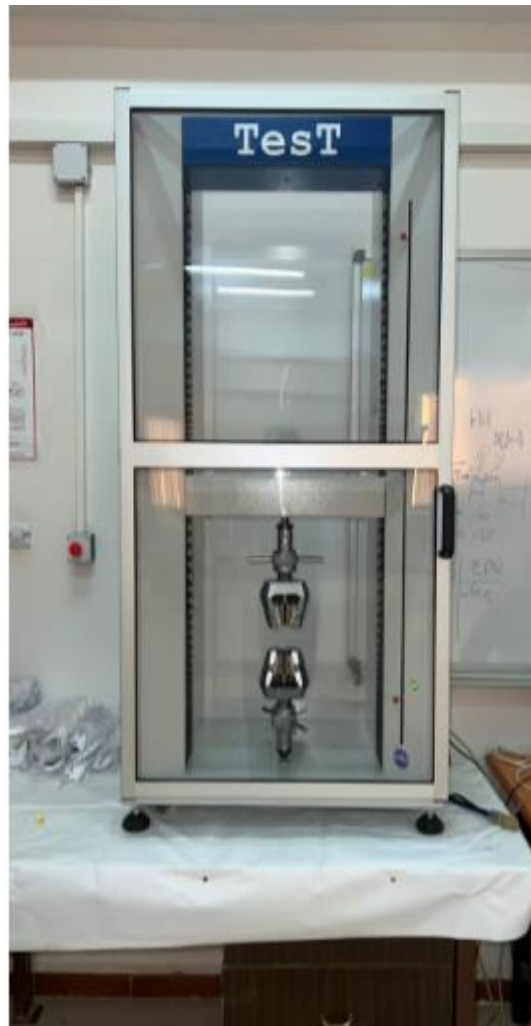
Figure II.7. Machine de traction de type TEST.
