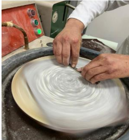
Figure 14.II.5. Machine de polissage.
