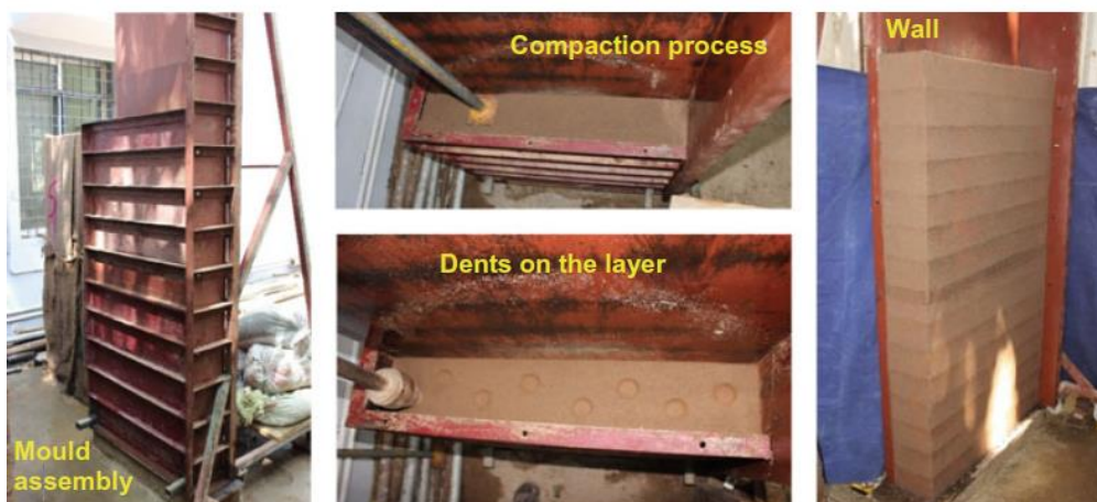
Fig20: Metal mould assembly, compaction process and CSRE wall specimen
