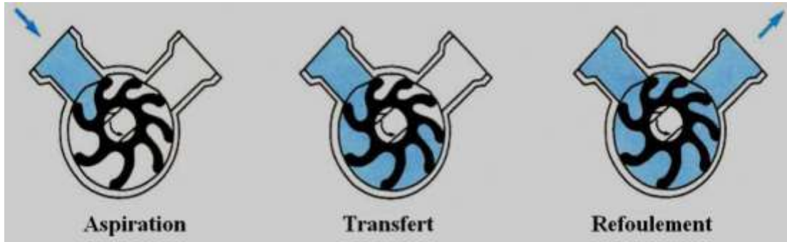
Figure II.6: Pompes à palettes flexibles. [14]
