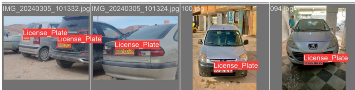
Figure 3.3 licence plate detection using Yolov8
