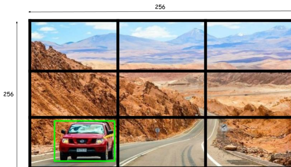
Figure 2.14 YOLO using Grid (3 \times 3)
