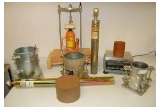
Figure II-9 Appareillage Essai Proctor
