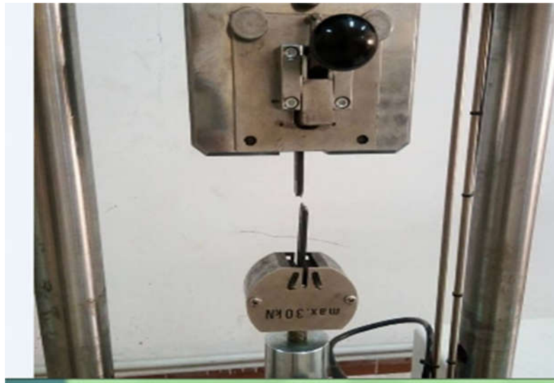
Figure III.8: Eprouvette subi un essai de traction
