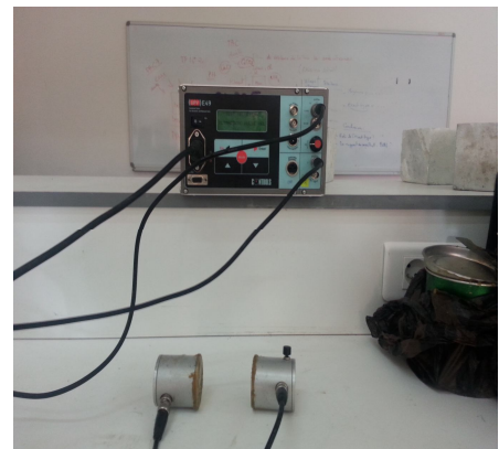
Fig III.6: Ultrasonic tester E 46
