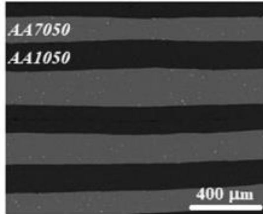
Figure I.4. Macrostructure of AA7050/AA1050 components processed with ARB [1].
