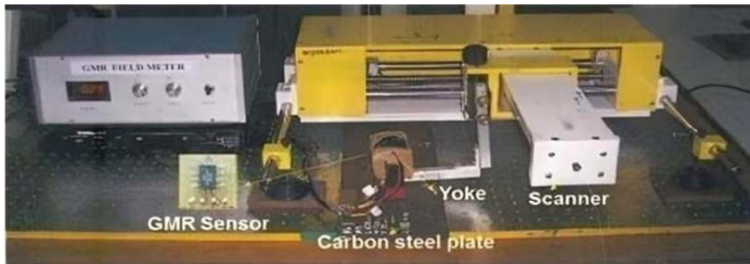
Figure 7: Experimental set-up for MFL measurements in carbon steel plates.
