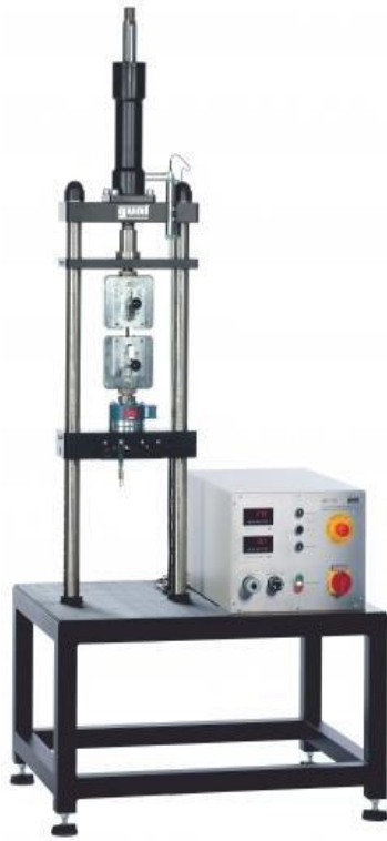
Figure 6 : Diagram of the traction machine.
