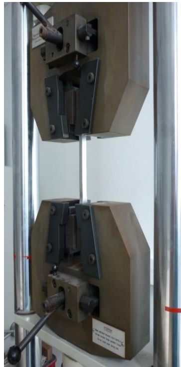
Figure 6 : Diagram of the traction machine.
