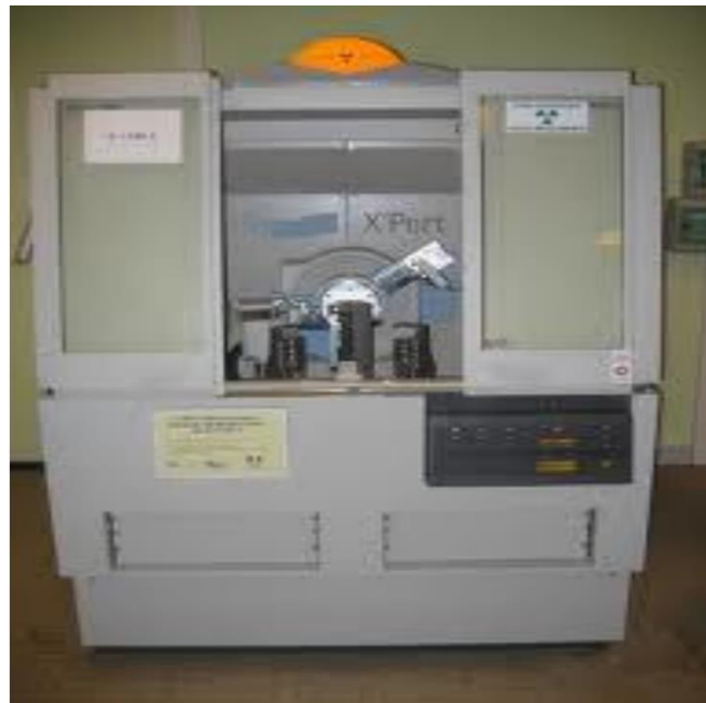
Fig. V.2: Image of X-ray Diffraction (XRD) apparatus used in our work.
