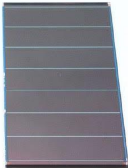
Figure II -5 : cellule photovoltaïque amorphe
