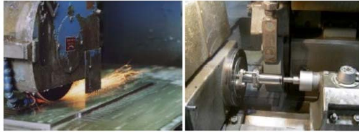
Figure II.6. Rectification plane et cylindrique, [4,5]
