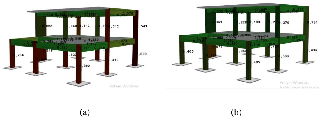
Figure 4.24. Members chord rotations of the Building strengthen by adding shear walls, a) For Damage limitation DL b) Significant damage SD.
