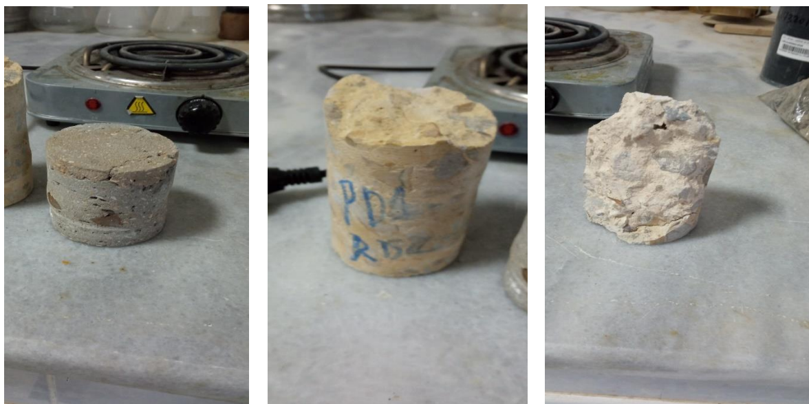
Figure 2.3. Concrete specimen after and before testing.
