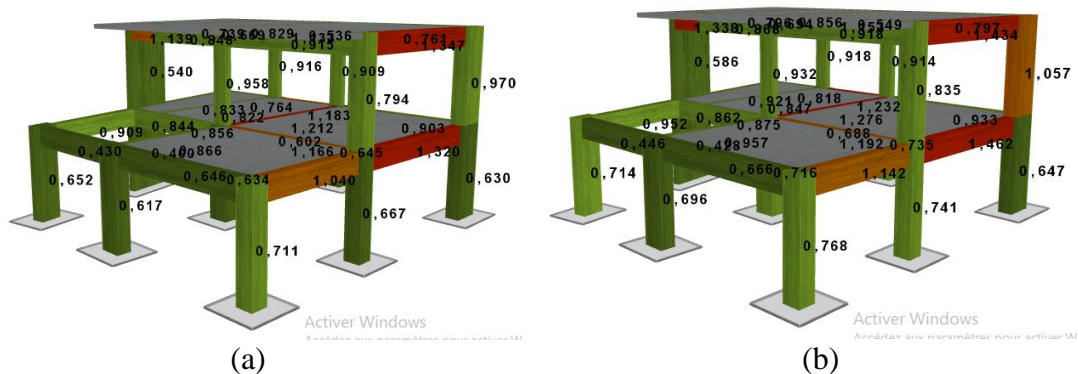
Figure 4.20. Members shear forces of the Building strengthened by elements jacking, a) For Damage limitation DL b) Significant damage SD.
