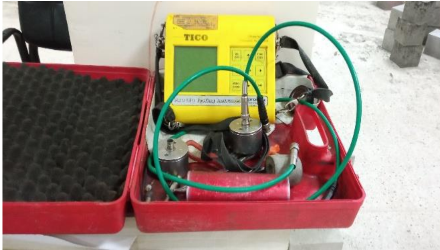
Figure 2.6. Ultrasonic Pulse Velocity (UPV).
