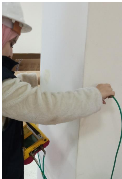
Figure 1.17 execution of UPV test.
