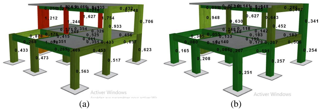
Figure 4.19. Member's chord rotations of the Building strengthened by elements jacking, a) For Damage limitation DL b) Significant damage SD.
