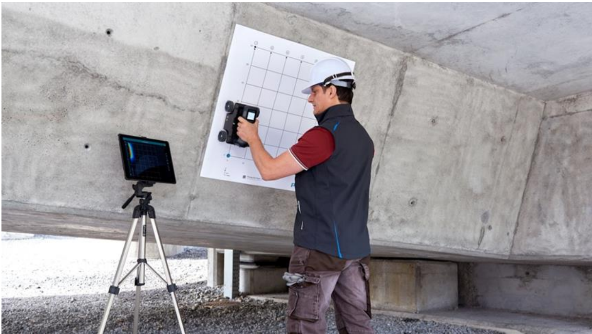
Figure 1.14 concrete rebar detection methodology [11].
