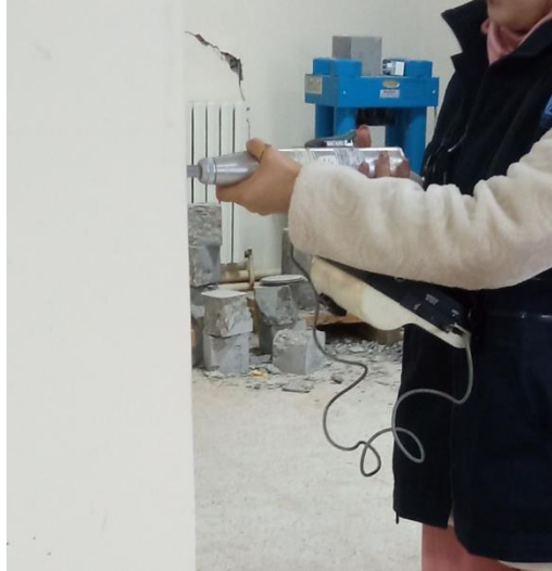
Figure 1.16 execution of a rebound hammer test.
