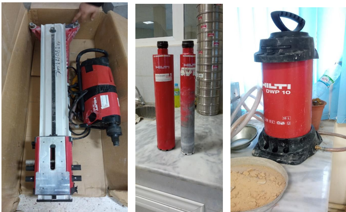
Figure 2.2. Rotary cutting tool.
