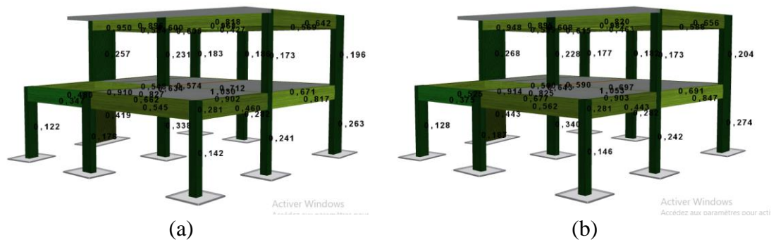
Figure 4.25. Members shear forces of the Building strengthened by FRP wrapping, a) For Damage limitation DL b) Significant damage SD.
