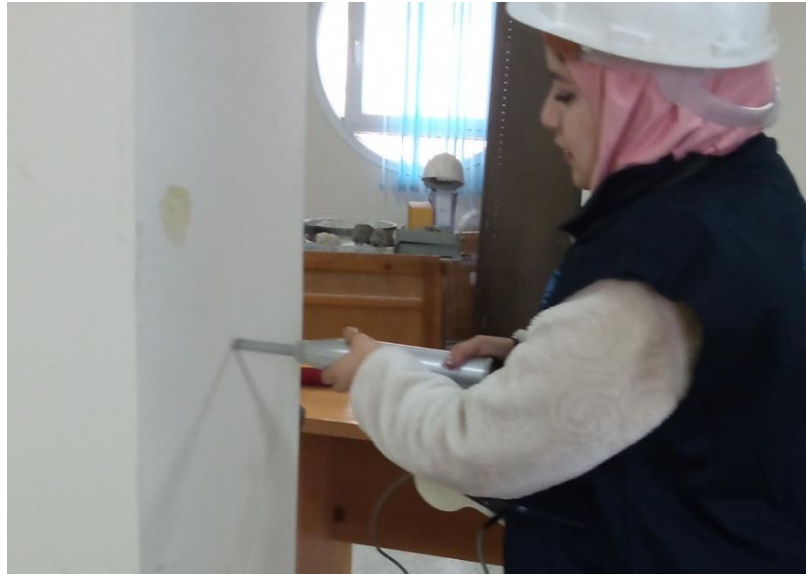
Figure 2.5 Test Procedures of Rebound Hammer.
