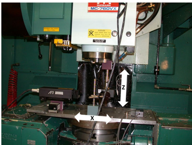
Fig. 4 Measuring setup on the Matsuura MC-760 VX machine tool using 5/6D API device
