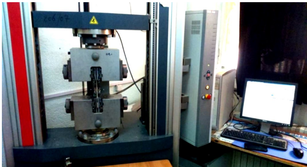
Figure III. 6. Machine de traction /compression Zwick- Roell type z100.
