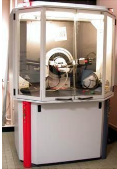
Figure II. 9: diffractomètre de type (D8 ADVANCE) [2]
