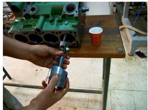
Figure II.55 : Remontage attelage mobile.
