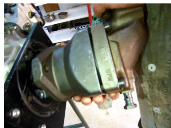
Figure II.67 : Remontage pompe hydraulique.
