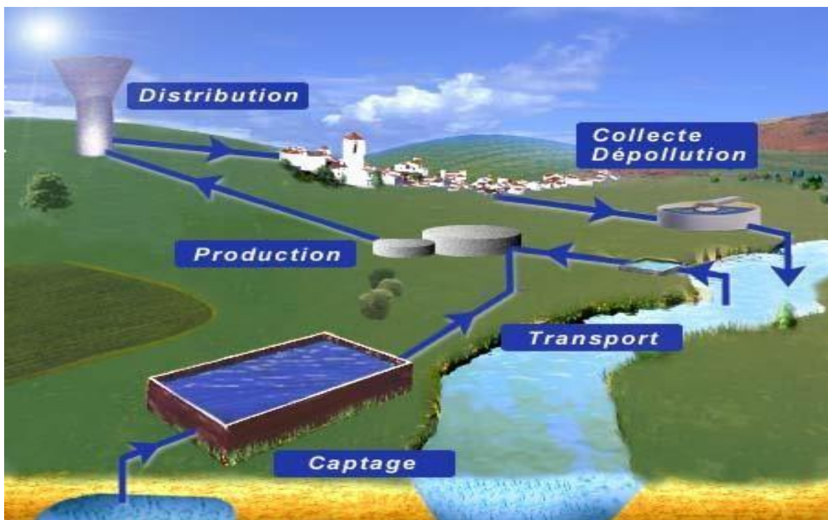
Figure I.1: le circuit de l'eau potable
