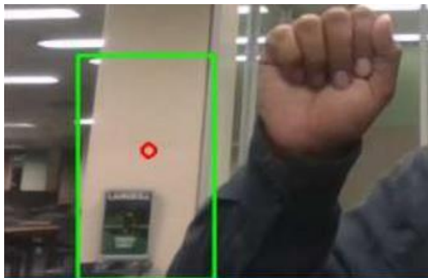
Figure 1-17 An Example of False Detection of Hand Region in Skin Based Detection Technique [7].
