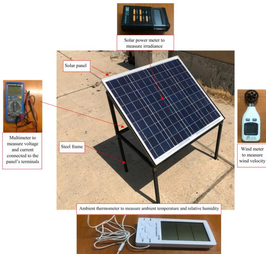
Figure I.20: Photovoltaic module and measuring devices used in the study of Sohani and Sayyaadi [110].
