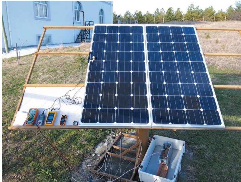
Figure I.18: Free-standing photovoltaic module and measuring equipments used the study by Ayan and Toylan [61].
