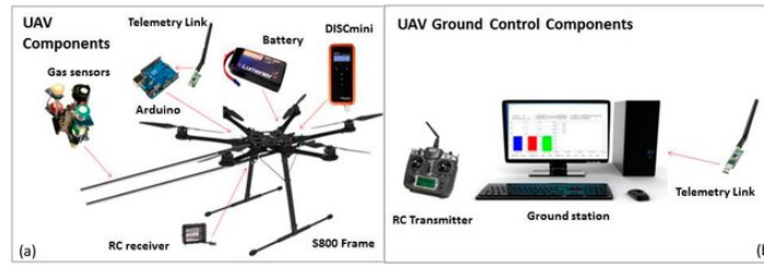
Figure 1.2: Components of a typical Unmanned Aerial System
