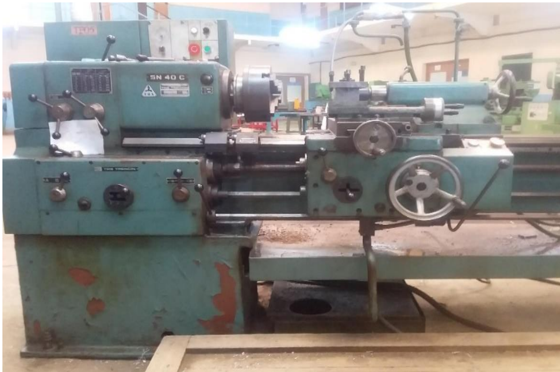
Figure V-1 :Tour conventionnelle SN40C
