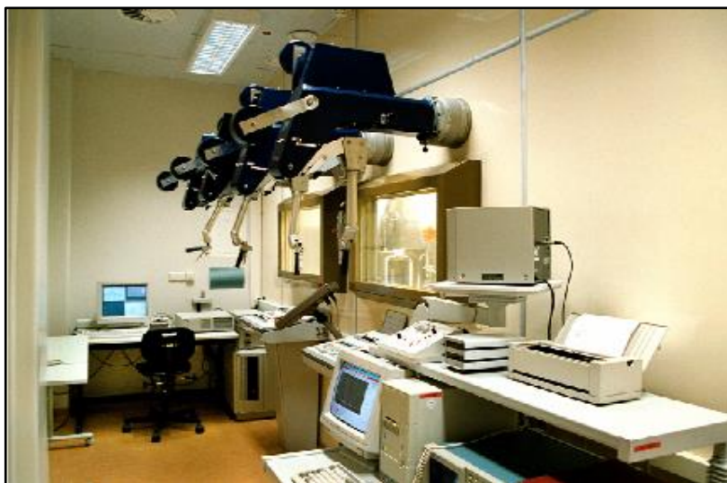
Figure 1.3: Hot cells with manipulators used for radioisotopes/radiopharmaceuticals production available from commercial sources. [13]
