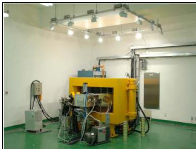
Figure 1.2: A 13 MeV cyclotron (indigenous product) in operation in Chosun University, Republic of Korea. [13]
