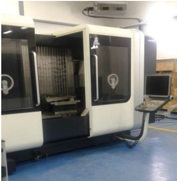
Figure IV 13: CUV 5 axes type DMG
