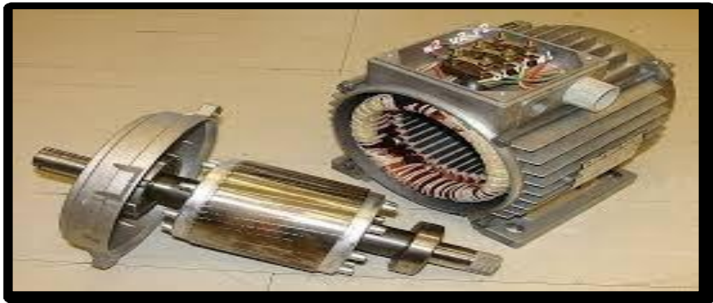
Figure I.1 : la structure de la machine synchrone a aimant permanent [FERA 22].
