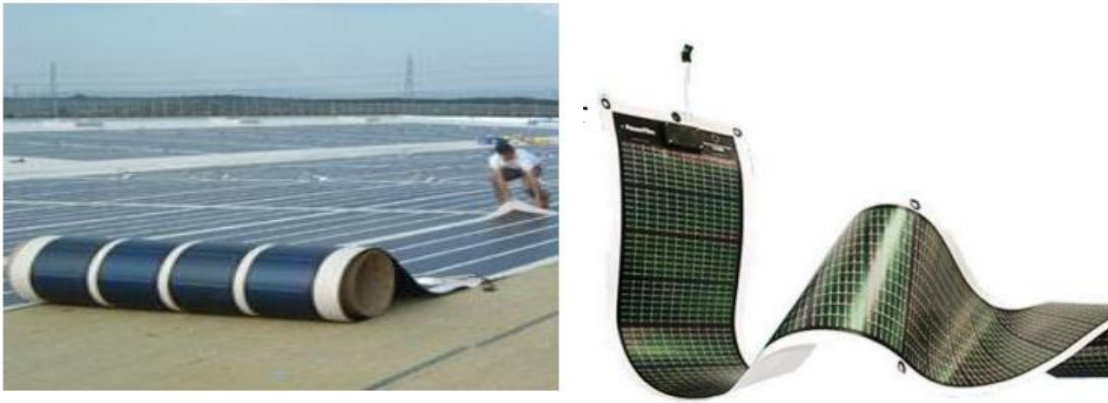
Figure (I-8) : Cellule type amorphe.
