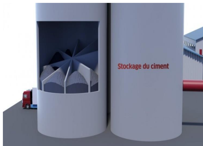
Figure III.14 : stockage du ciment
