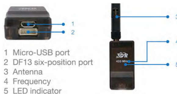
Figure II.14 Telemetry hardware description
