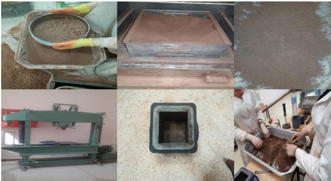
Figure IV.11: processus de confection de BTC.
