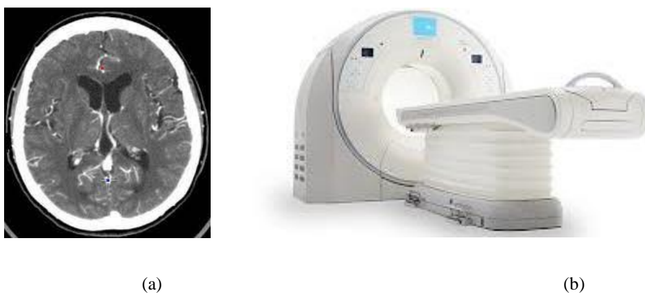
Figure I.2. Computer tomography (CT): a) CT brain image and b) CT scanner.
