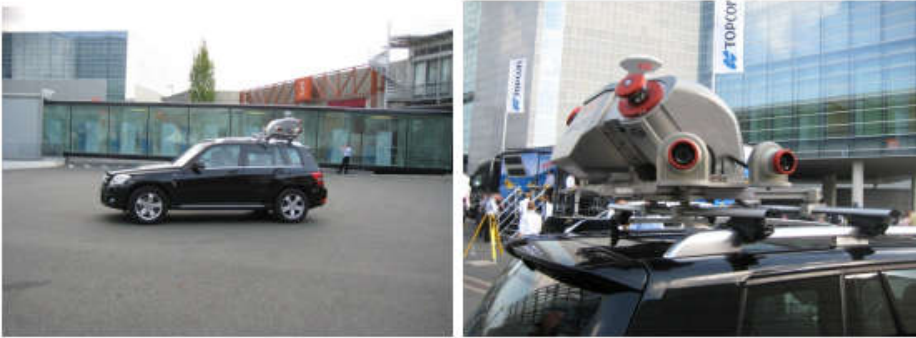
Figure 6 car- borne mobile scanning system
