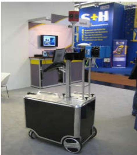
Figure 5 small-vehicle-borne mobile scanning system
