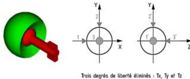
Figure II. 11: La liaison rotule
