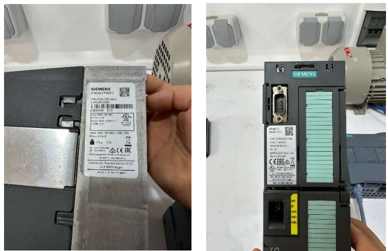
Figure 27 Siemens SINAMICS G120 Control Unit 240E-2PN with PROFIBUS DP Interface
