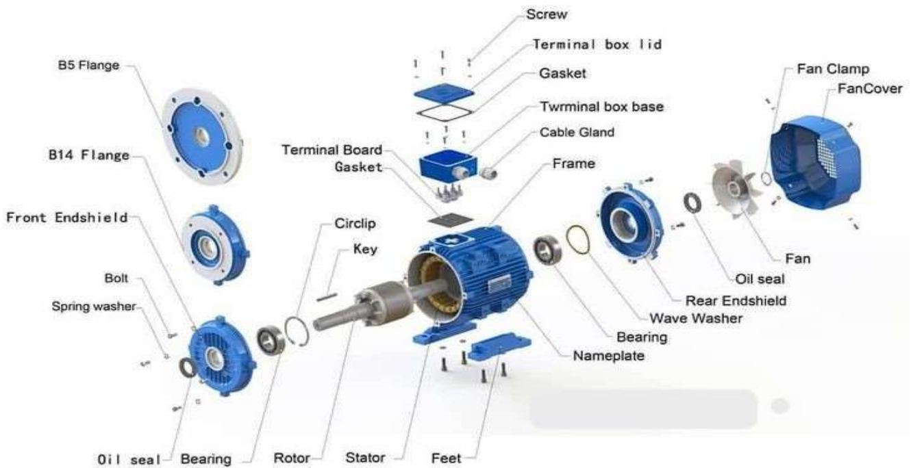
Figure 19 Diagram of the components of an asynchronous machine
