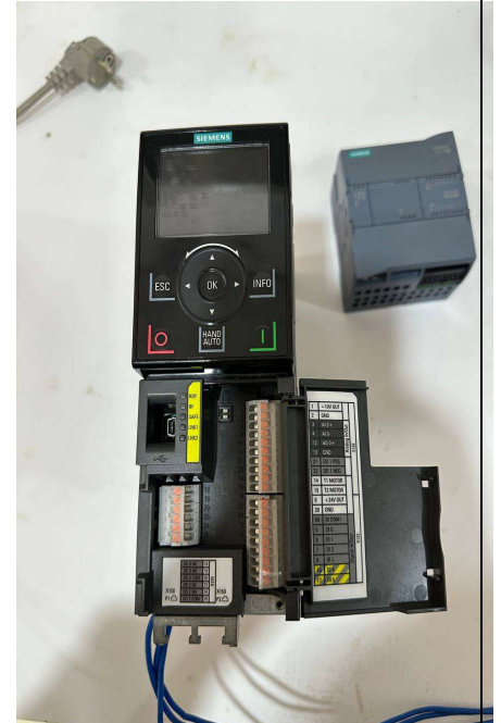
Siemens SINAMICS G120 Power Module and Basic Operator Panel (BOP-2)
