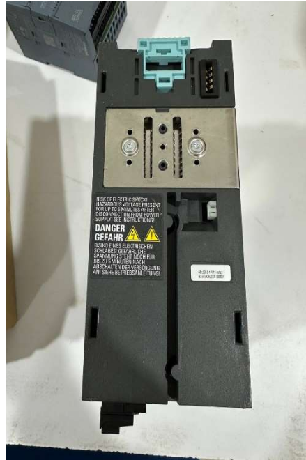
Siemens SINAMICS G120 Power Module and Basic Operator Panel (BOP-2)
