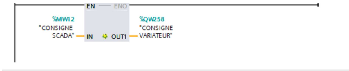
Figure 41 Siemens TIA Portal LAD Program for Motor Stop and SCADA Setpoint Control
