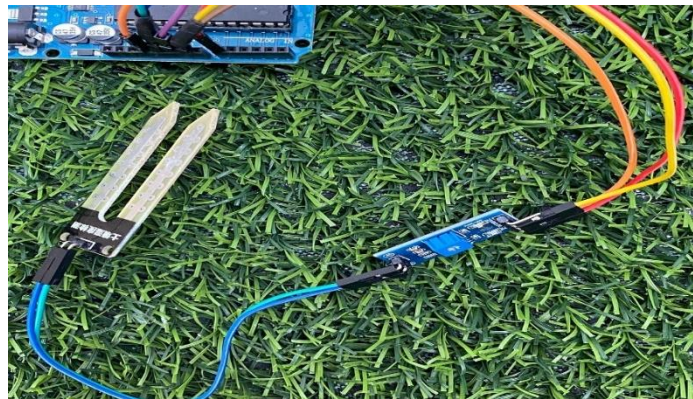
Figure 3.12: Soil moisture sensor placement
