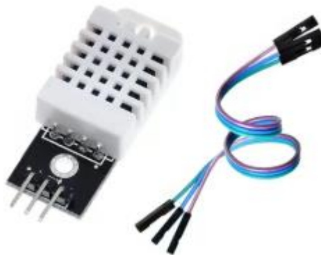
Figure 3.2 :DHT22 Temperature and Humidity Sensor
