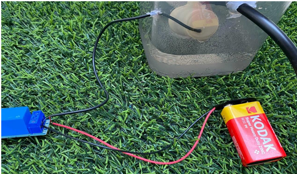
Figure 3.15: Pump connected through the relay
