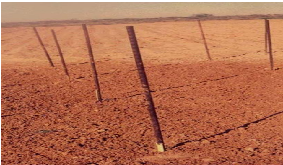
Picture 16: The stake method used in the lands to quantify the eolian erosion
