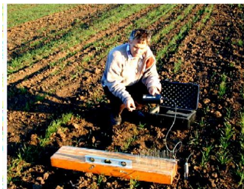
Picture 06: Roughness tester (according to Nord, 2006)
