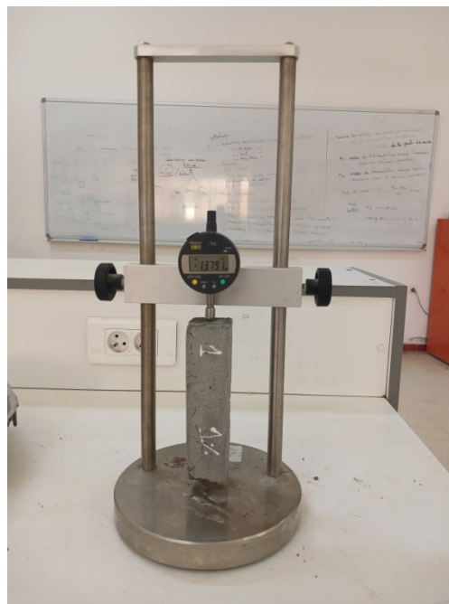
Fig III.26: Essai de retrait
