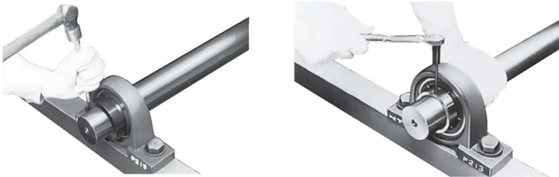
Figure III.6 Fixation des paliers
