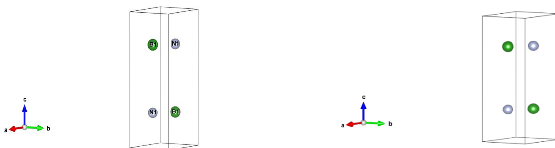
Figure (III.1): The crystal structure of Boron-Nitride h-BN in 3D.
