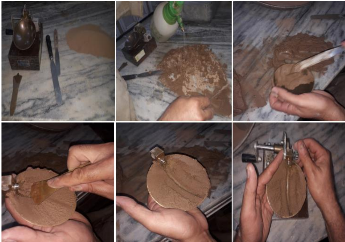
Figure II.12: Steps follow to determine Atterberg limits
