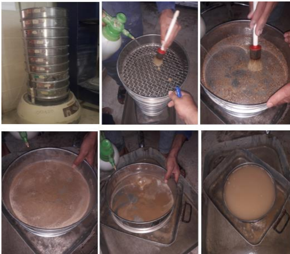
Figure II.7: Steps follow to determine grain size sieve
