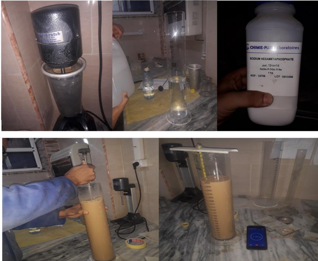
Figure II.10: Steps follow to determine hydrometer grain size sieve
