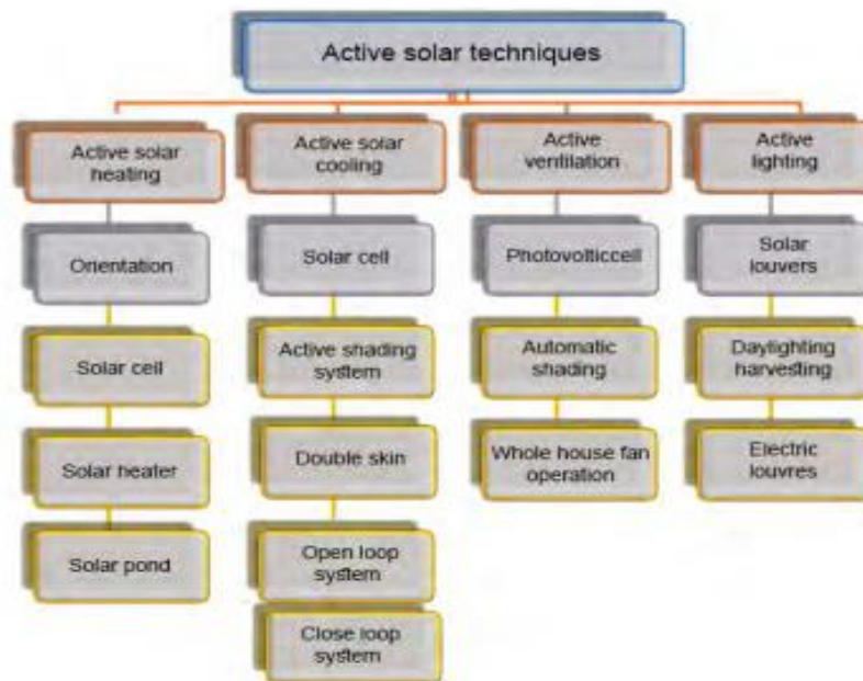
Figure I.19:3 Strategies for using active solar to reduce energy consumption inside buildings [27]
