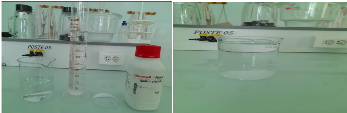
Figure 11: Solution corrosive de NaCl de 0,2 M
