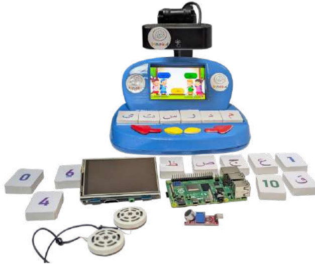
Figure 3.14: Functional prototype of the InnoKid interactive educational device utilizing camera vision and physical interaction
