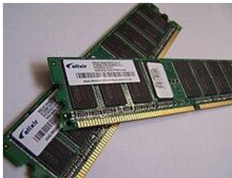
Figure 1.3 : Two DDR memory modules, each with a capacity of 512 Mb
