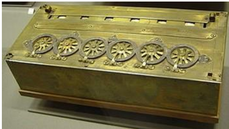
Figure I.1 : A Pascaline, the mechanical calculator invented by Blaise Pascal in the 17th century, on display at the Musée des Arts et Métiers in Paris. This device could perform additions and subtractions and is one of the first examples of a computing machine.
