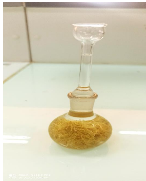
Fig II.8 Pycnometer used for density measurement.
