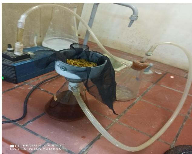
Vacuum filtration of cellulose
