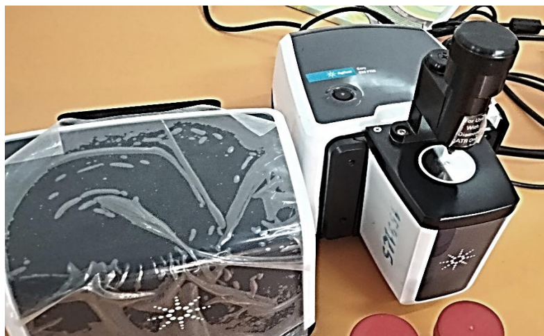
Fig II.5 ATR-FTIR device used for fiber spectroscopic analysis.
