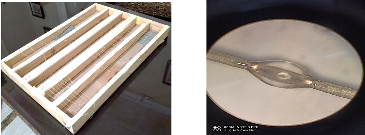
Fig II.11 Preparation of polyester microdroplets on treated and untreated Alfa fibers.
