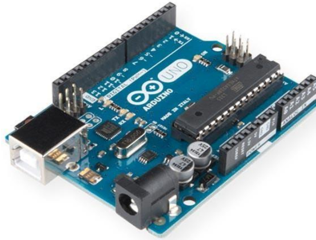
Figure 1: An Arduino Uno board with its connectors.
